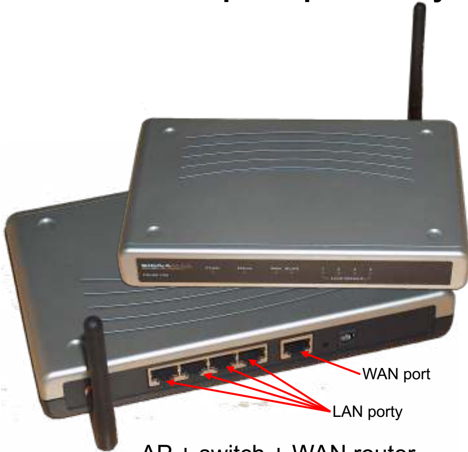
AP + switch + WAN router
