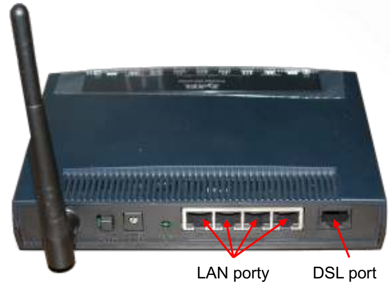
AP + switch + DSL router
