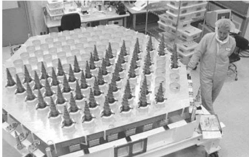
Figure 6.10 A 120-element Inmarsat-4 satellite L-band feed array being assembled Antennas for Cellular, Multiple-Spot-Beam Coverage
