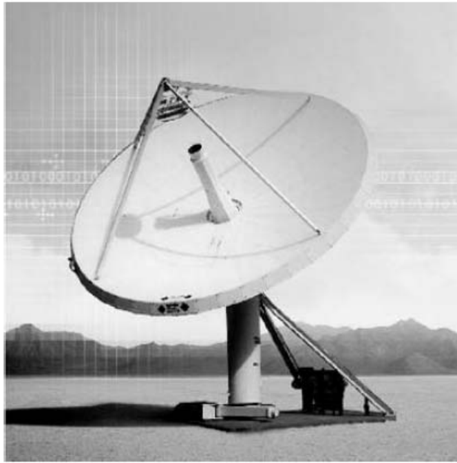
Figure 6.12 An example 9 m cassegrain ground station antenna.
